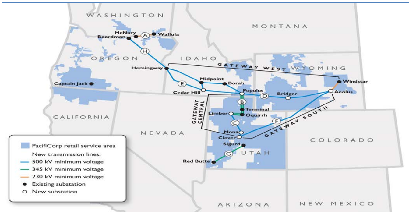
Figure 1: Energy Gateway Transmission Expansion Plan
